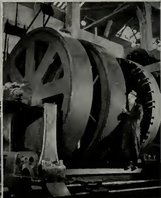
Center below: View of the Mobilube on drydock at Bethlehem's San Francisco Yard. Upper half of temporary planking of "soft patch" has been removed revealing temporary frame. Lower right: Mobilube's huge reduction gear being inspected in Bethlehem's machine shop.
